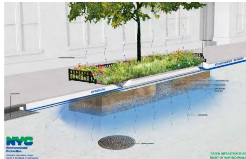
Schematic Sketch of Right of Way Bioswale
